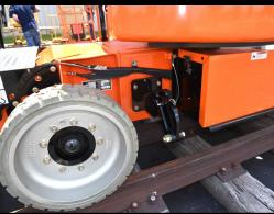
Model 1010 WTC Flexiride® Rail Gear has 4-wheel independent torsion suspension that self-compensates for uneven track conditions. The basic system is provided with a self-contained hydraulic power unit with emergency hand pump, front and rear rail sweeps and external push button controls.
