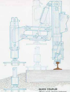
Allows quick change between standard bucket and specialized One Man Gana attachments
