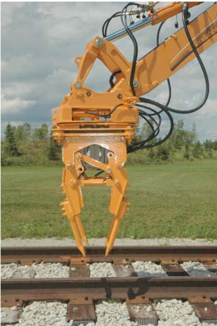
The Tamper is capable of tamping one side of the tie at a time. A production rate of 60 ties per hour (Single Squeezes) can be achieved.
