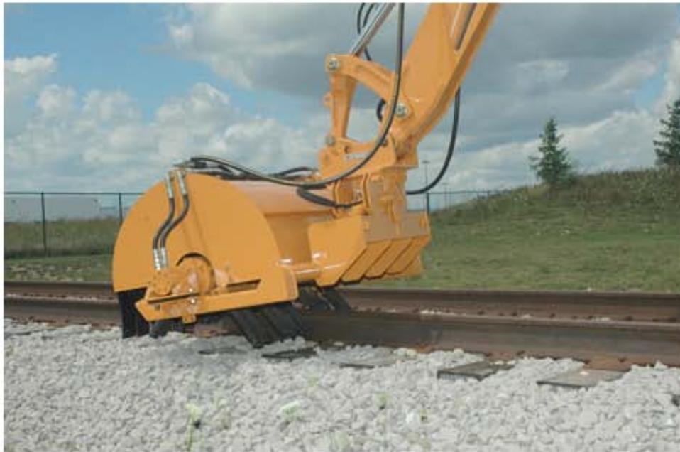
The Ballast regulator can be positioned to either go down the center, over each rail or rotate tilted over the track shoulder.
