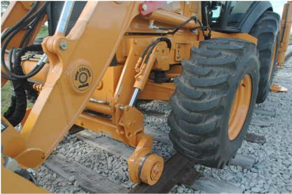
The front Rail Gear bolts to the front backhoe frame through an adapter plate that is welded to the front frame.
