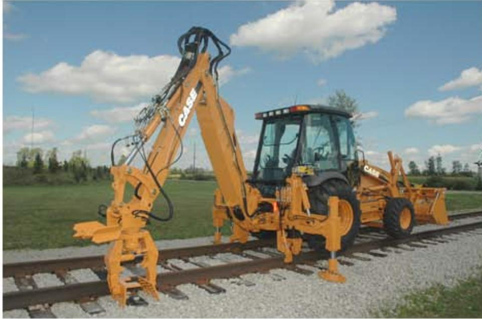
The Attachment used to remove in insert railroad ties is the 360° rotating Tie Head.
