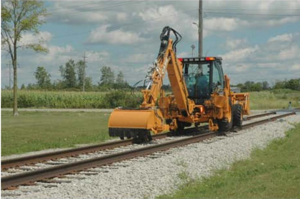
The Attachment used to regulate the ballast on the ties and track shoulder is the Ballast regulator.
