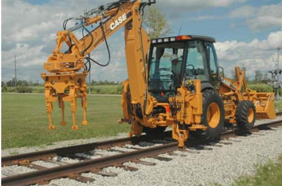
The Attachment used to tamp the ballast under the tie is the Tamper.
