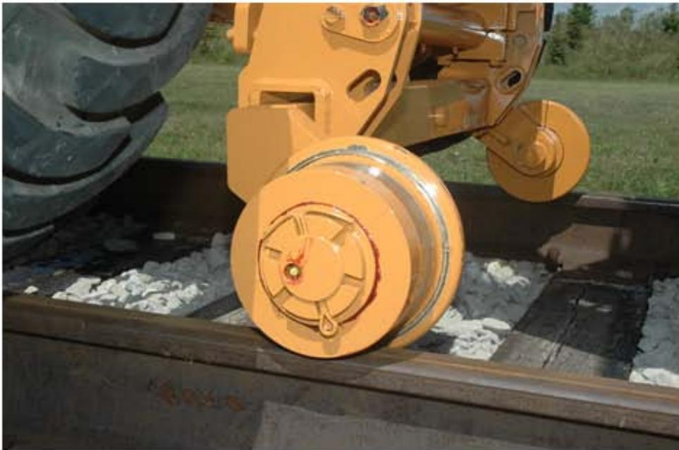
The front machine axle is spring loaded to stay level as the backhoe self-propels down the track.
