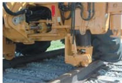
Standard features include 8 inch hardened steel rail wheels with heavy duty Timken bearings and independent suspension that will compensate for uneven track conditions.
