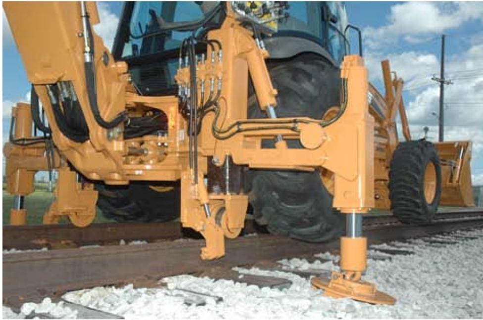
The rear Rail Gear pins where the standard backhoe wing down stabilizers were attached to the backhoe frame.
