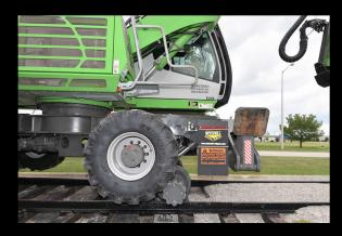
Mitchell Friction Drive for Rubber Sennebogen Material Handlers allows the machine to self-propel on the railorad track to work on rail or work on the ground with the friction Drive Hi-Rail Gear retracted. The configurations allows the outriggers to remain on the machine for working on the ground. Optional extended outriggers legs available.
